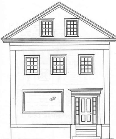
↑ **Inappropriate** Enlarged window opening for picture window.
