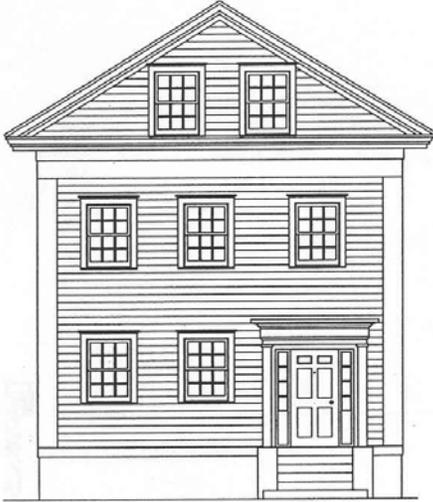
↑ **Appropriate** Original narrow clapboards, typically 3"- 4" of exposure.
