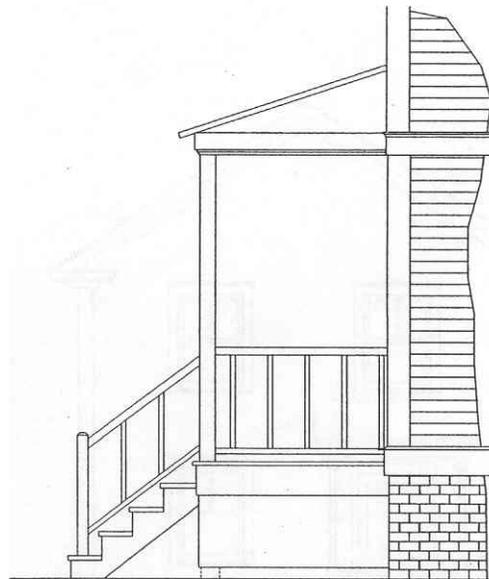
↑ **Inappropriate** Balusters are too far apart. No visual support for column. No cap on railing post. Lack of molding on roof. Lack of detail on column.
