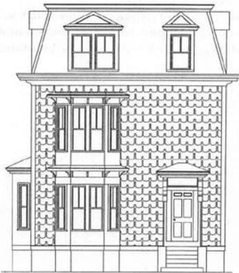
← **Inappropriate** Asphalt shingles, window filled in.
